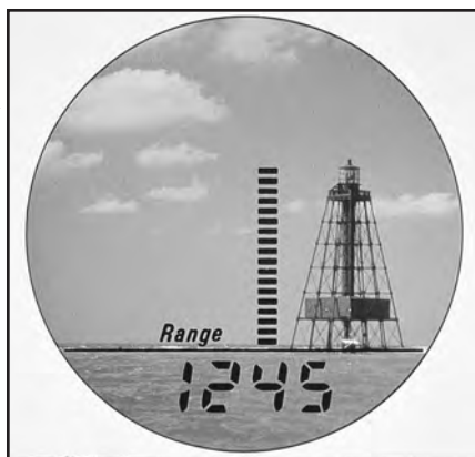
FIG. 4-4 —Use of KVH Datascope® to Measure Range from Object of Known Height
