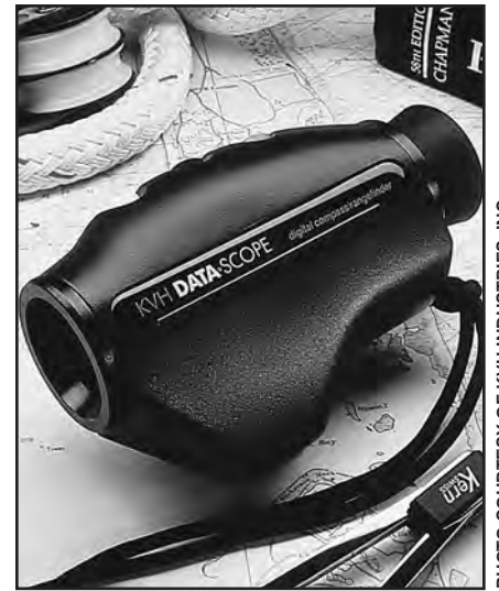
FIG. 4-3 —Handheld monocular (KVH Datascope®) combines a fluxgate compass, timer, and range finder.
