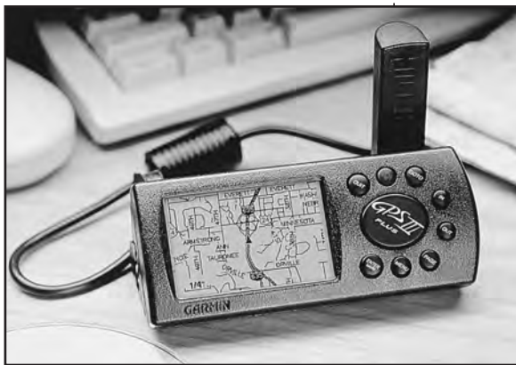
FIG. 4-13 —Another Handheld GPS Unit with Navigation Database
