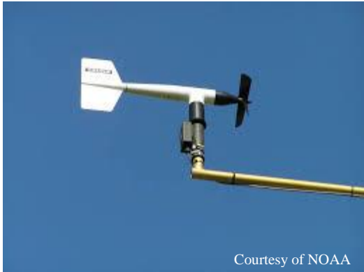
Figure 2.12. A typical anemometer, with a propeller for measuring wind speed.
